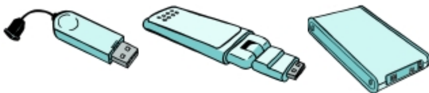
A USB memory stick, a wireless antenna and a USB hard drive that plugs into a USB plug on a laptop or a PC.
